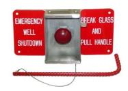
The **16RS48** is a glass enclosed, stainless steel, Emergency Shutdown (ESD) Station with easy-view large letters and a red background. It has a 1.00 Inch Diameter panel hole for installation of either the 16RS36 (2W-N.C.) or 16RS40 (3W-N.O.) ESD Relay valve.
